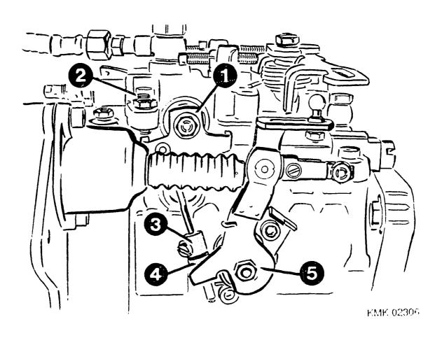
1 = Cylindrical helical coiled spring
